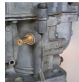
4-mm hole, and cutting M5-thread into the dual choke carburettor (see photo) because these are already prepared for a vacuum nipple. The nipple is supplied with the 123\EVO.
